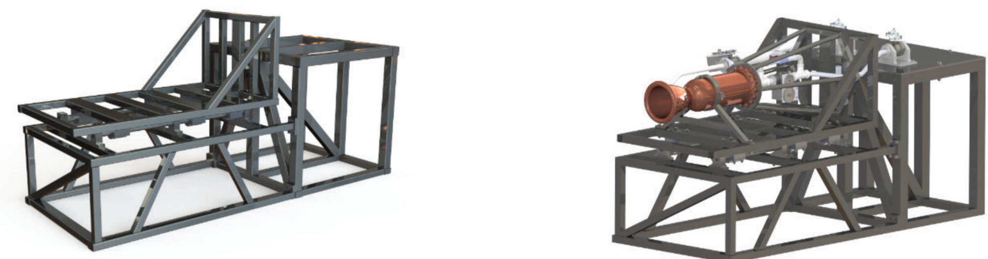
Figure 4. Final design of the new testing equipment with application example for liquid propellant motor.
