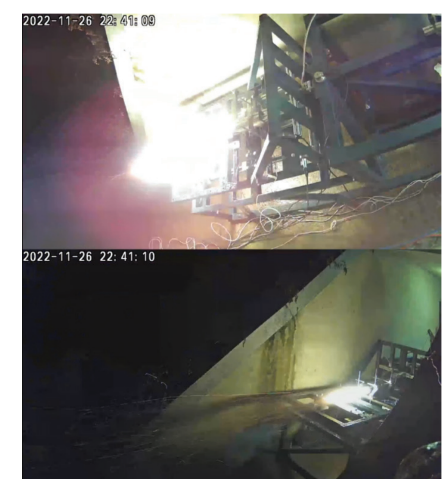
Figure 8. Frames from the IP cameras – idle test setup (left), engine during test (right).
