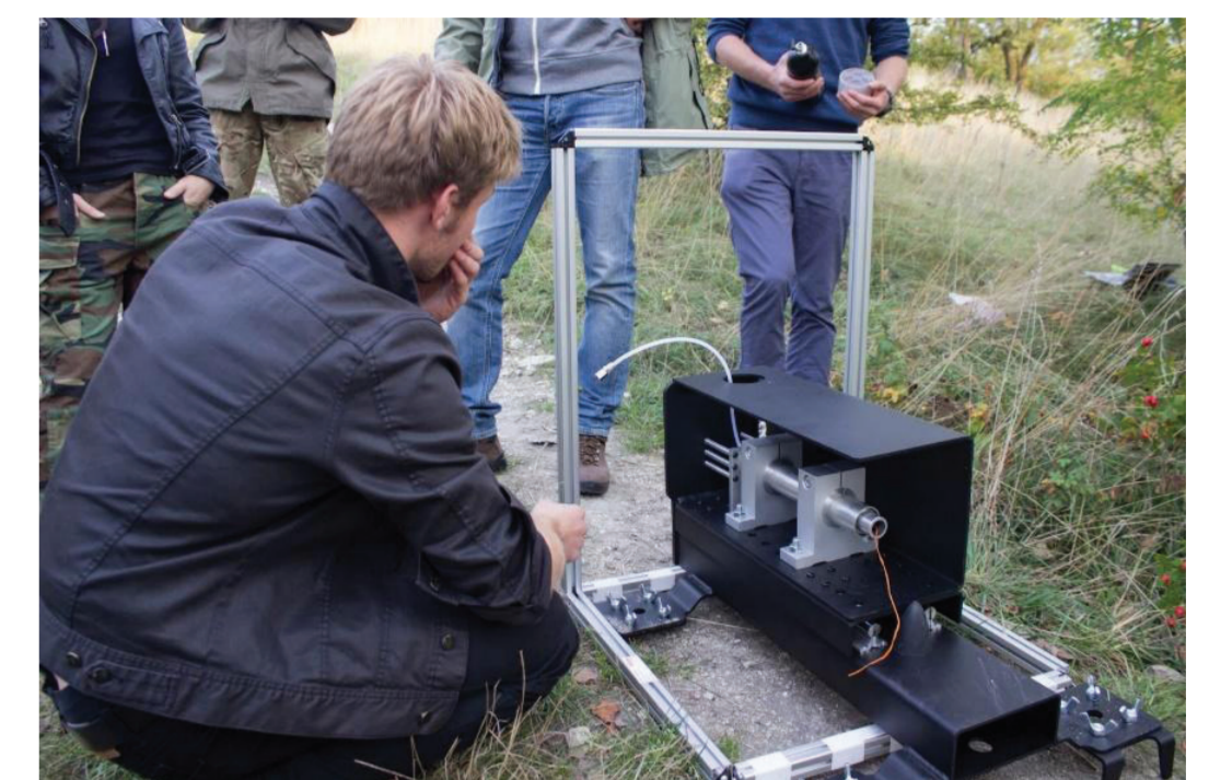
Figure 1. First test stands for rocket motors manufactured by AGH Space Systems.
